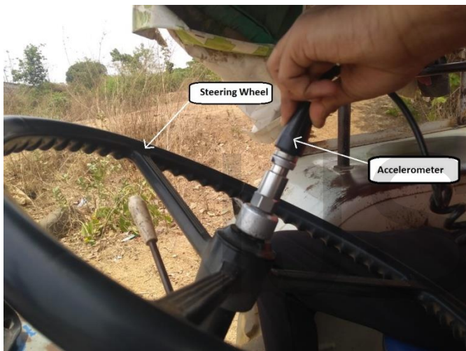
Fig.1. Accelerometer mounted on steering box
